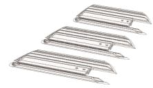
4. Insert X-Bracket assembly into the end of the Sliding Rail and tighten down screws
