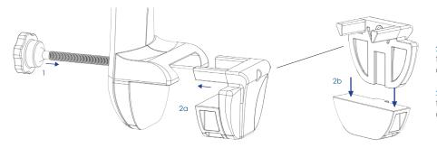
2a. If using the RMS on a rimmed tank; leave the included spacer on the clamp chop.
