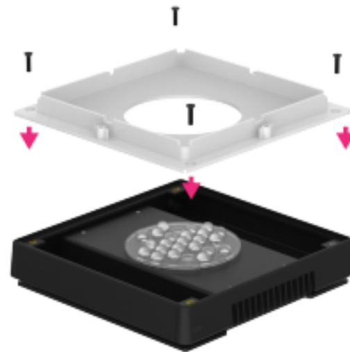
Place the reflector on to the light assembly.
