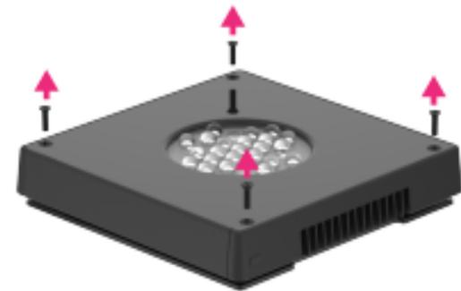
Remove the four corner screws from the lens frame.
